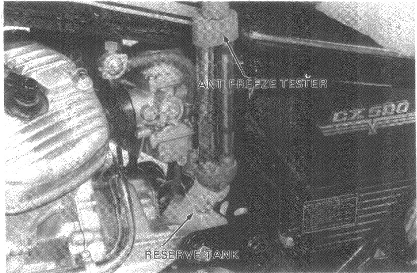
COOLING SYSTEM TESTER M988X-525-XXXXX
